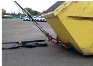
Ballast weights and tanks function as a reliable anchor on tarmac-covered squares.
