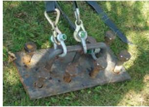
Floor slabs and ground anchors with a length of 1.00 meter each. This requires a previous verification using layout diagrams to determine if underground cables are present in the area concerned.
